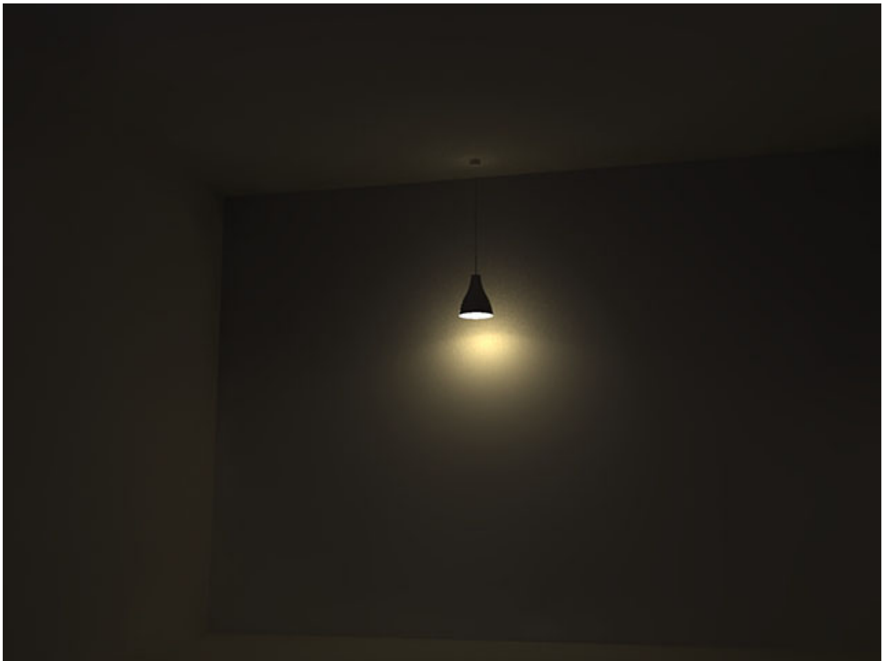
Figure 17 - Rendered view of the modified fitting showing the scalloped pattern on the wall
