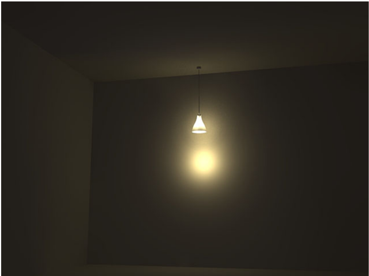
Figure 22 -Rendered example of omni light 'burnout' when the light is too close to a neighbouring surface
