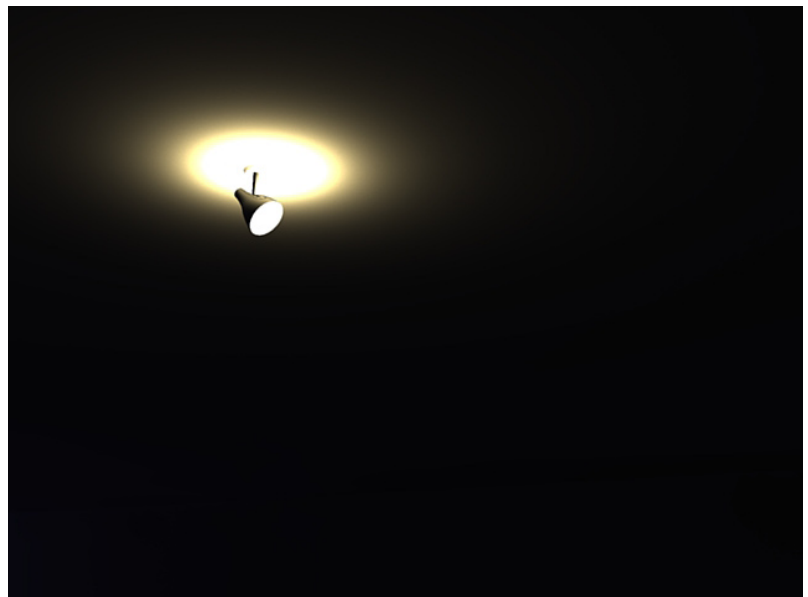
Figure 23 - The effect of locating omni lights inside small fittings close to neighbouring surfaces at minimum strength.
